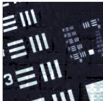
512 x 512 image constructed using multi-pixel compressive sensing from a 64 x 64 sensor.
